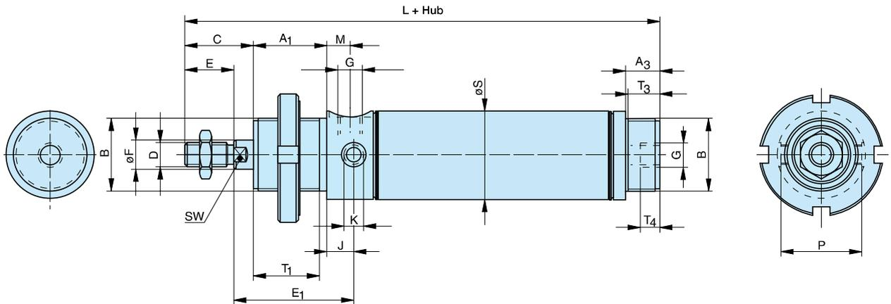
Abmessungen (mm) – Basic Zylinder, Serie R..., RK..., RDU...
