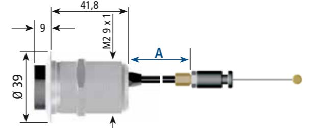
Protruding push-button with lateral bowden cable exit
