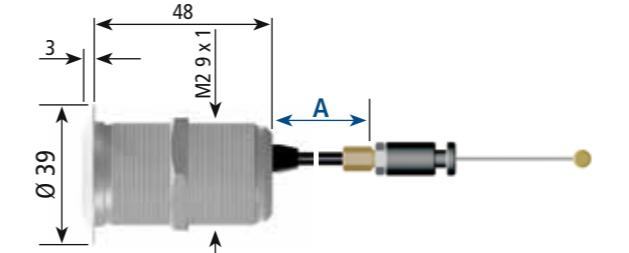
Flush push-button with lateral bowden cable exit
