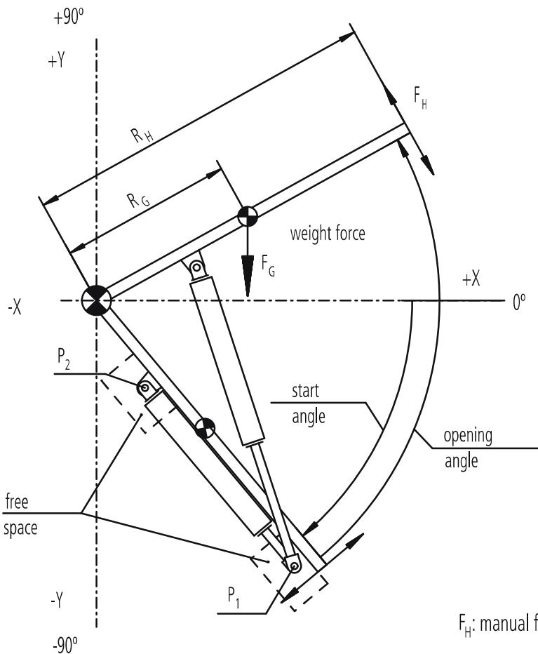
STABILUS recommends a minimum manuel force of 20 N at -30° C at open position. Is the calculated manuel force below 20 N, the agreement of the customer is needed.
